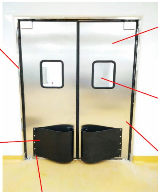
1.0mm 304 oil ground stainless steel wire drawing plate is used for the surface of door panel. The core material is XPS extruded board, which conforms to GB8624- 2012 standard and has the functions of heat preservation, waterproof and heat insulation.
